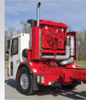
Remote Mounted Radiator
